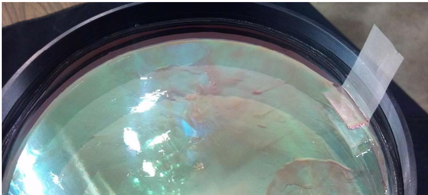
Here is the lens partially coated with polymer with the oring acting as a dam to stop the polymer flow. Chemical resistant mesh (FCNet) is embedded in the partially dried polymer as a handle to peel once dry
