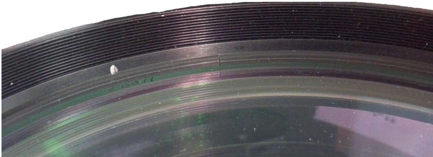
Here is an oring placed around the perimeter of an 8"D Studio-style lens with ends butted together at the 12-o-clock position
