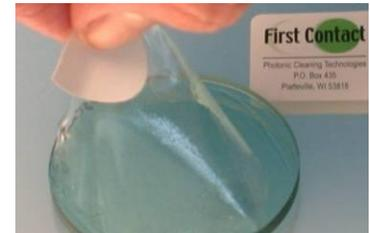
The solvent system has been carefully developed to work with high quality optics, mirrors, and diffraction gratings. The solvents have been selected to dry at a controlled rate, avoiding thermal coating stress which could ruin the optic. The system is quite safe, utilizing common solvents like ethanol and acetone.
