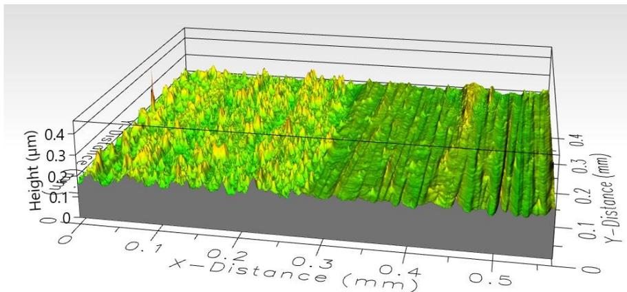
In this white light interferometry data, the Z scale (height) is 1/10<sup>th</sup> micron. First Contact Polymer was applied to the right half of this diamond turned copper substrate, allowed to dry, then peeled. One can clearly see nanoscale particle profiles on the left half of the image (uncleaned) and the substrate's actual surface texture in the right half (cleaned). All contamination was removed and the surface left pristinely clean. Data courtesy of Photonic Cleaning Technologies 3/2020
