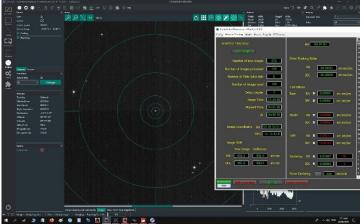
Adaptive tracking software I wrote to provide precision tracking during an imaging run. ATrack is used to maintain the star in the center, much like an autoguider.
