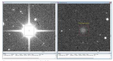
Ghosting is an artifact of sCMOS cameras where the pixels can retain charge after clearing for a short period of time. The image on the left is a bright star before a pier flip and the image on the right is after the pier flip which moves the star to the opposite side of the image but shows the decaying charge still on the pixels. network database server for future reference if required.
