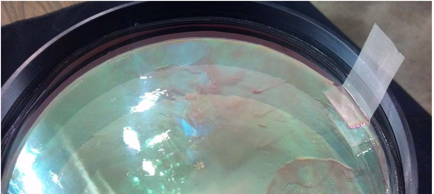
Here is the optic partially coated with polymer with the oring acting as a dam to stop the polymer flow. Chemical resistant nylon mesh (FCNet) is embedded in the partially dried polymer as a handle to peel once dry
