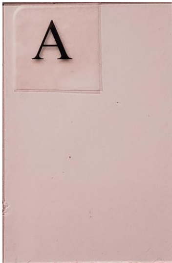
This color represents a dry film that's probably too thin to properly clean
