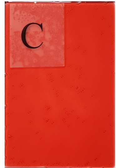
This color represents a dry film thickness to remove heavy contaminants and oil or grease residue
