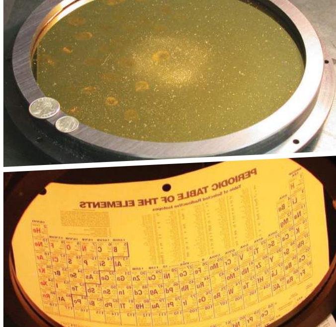
12 inch gold telescope spectrometer mirror restored to pristine condition in minutes.
