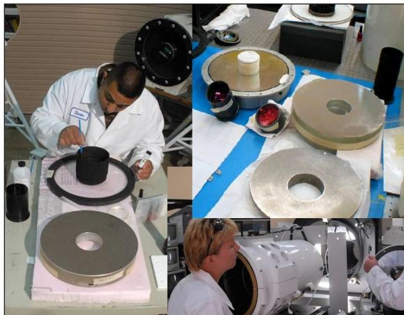
The WRDOG staff protects **Mirrors and Corrector Plates** with the polymer solution. Clean components from several telescopes are protected from recontamination while waiting for telescope assembly. Technicians may work without gloves until the film is removed after the mirror is placed in the telescope.
