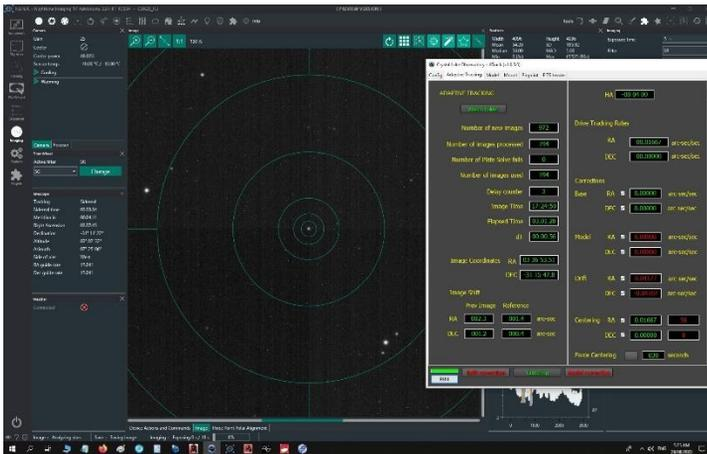
Adaptive tracking software I wrote to provide precision tracking during an imaging run. ATrack is used to maintain the star in the center, much like an autoguider.
