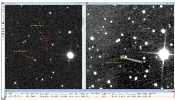
The image on the left shows two faint asteroids passing through the target field. Notice the CDK20 can reach down to 22 magnitude with a 3 minute exposure. The image on the right is a 3 hour composite showing the two asteroid trails.
