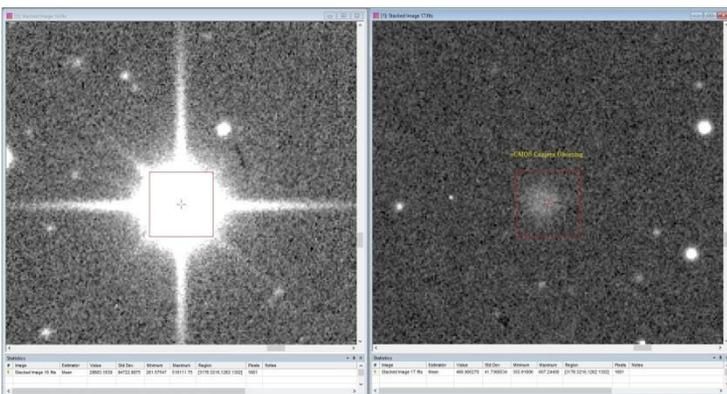
Ghosting is an artifact of sCMOS cameras where the pixels can retain charge after clearing for a short period of time. The image on the left is a bright star before a pier flip and the image on the right is after the pier flip which moves the star to the opposite side of the image but shows the decaying charge still on the pixels.
